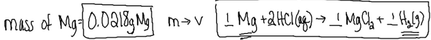
$$0.0218 \text{ g Mg} \times \frac{1 \text{ mol Mg}}{24.31 \text{ g Mg}} \times \frac{1 \text{ mol H}_2}{1 \text{ mol Mg}} \times \frac{22.4 \text{ L H}_2}{1 \text{ mol H}_2} = 0.0201 \text{ L H}_2$$
