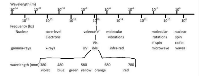
wavelength (λ) is equal to the speed of light (c) divided by the frequency (v)
