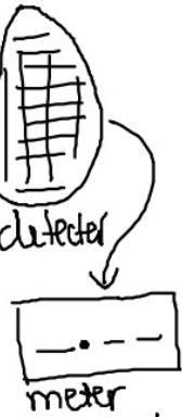
Energy from a variety of sources like flames + electricity used to excite  $e^-$  in the material. Because  $e^-$  will not stay excited energy is released when they return to a lower state, this energy is measured + reported as emission. emission spect.
