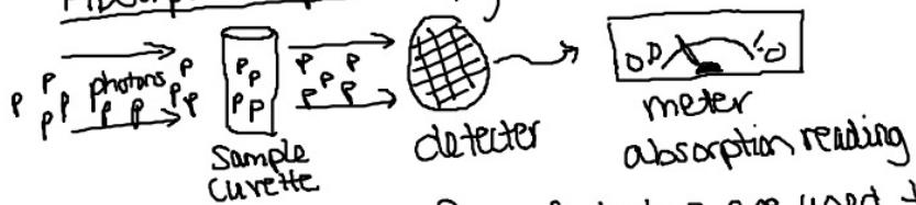
Light energy in the form of photons are used to excite the particles of materials, if the energy of the photon matches the energy required for the  $e^-$  to become excited the photon will be absorbed. The lack of the returning photon is measured + reported as absorbance.
